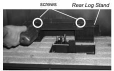
8) Remove the 2 screws & sleeves on the bottom brick panel and lift out the bottom brick panel. The brick panel is very fragile - handle with care.
